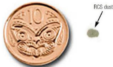
New Zealand 8 hour shift limit of Respirable Crystal Silica—you are at risk if you breath in more than this over an 8 hour period
